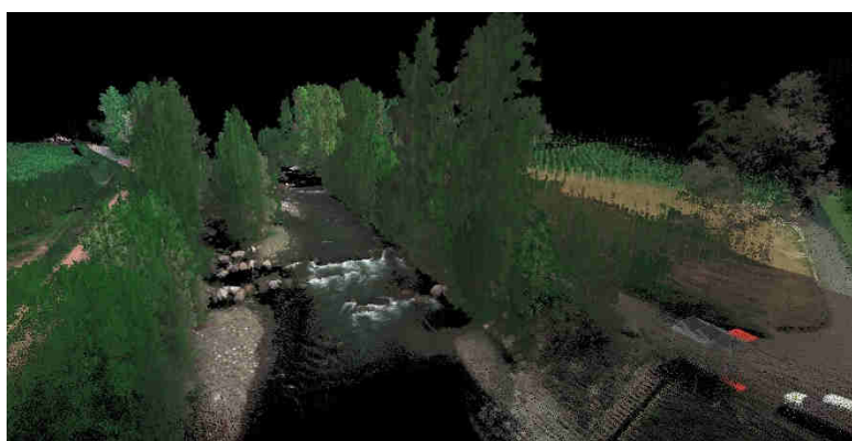
Figure 2 - LiDAR point cloud collected by RPAS survey
